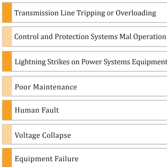
Figure 7.6. Causes of Power Blackouts
